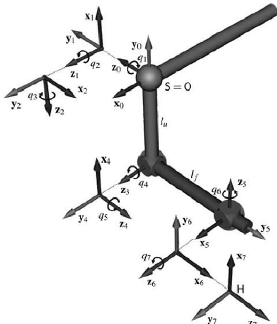
Figure 4: Simplified human arm kinematics using 7 DoFs
