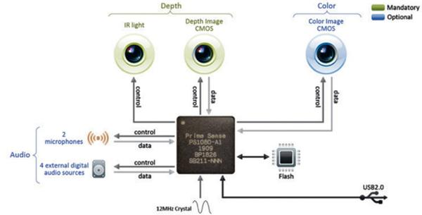
Figure 2: Kinect Sensor Diagram [15]
