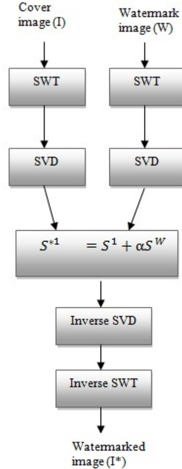
Figure 2: Block Diagram of the proposed watermark embedding algorithm
