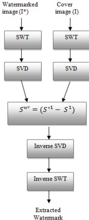
**Figure 3:** Block Diagram of the proposed watermark extracting algorithm
