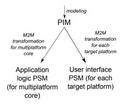
Figure 2: An overview of the approach to multiplatform mobile application modeling.
