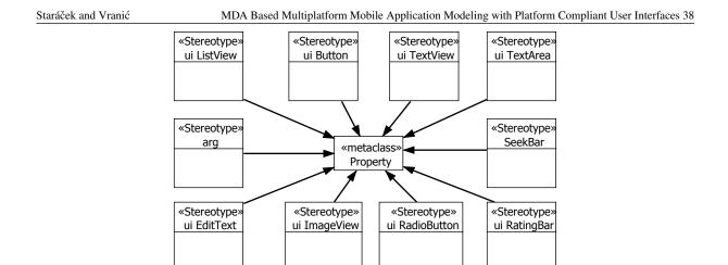
Figure 6: The UML profile with stereotypes applicable to the Property UML metaclass instances.
