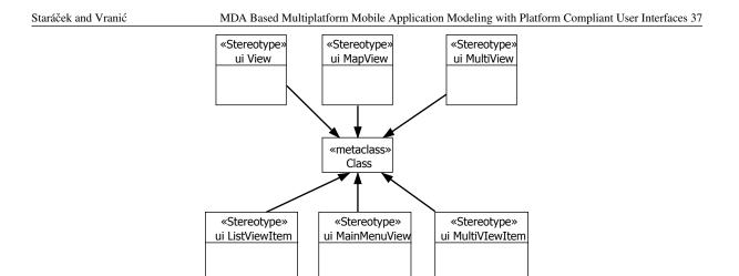
Figure 4: The UML profile with stereotypes applicable to the Class UML metaclass instances that constitute the user interface.
