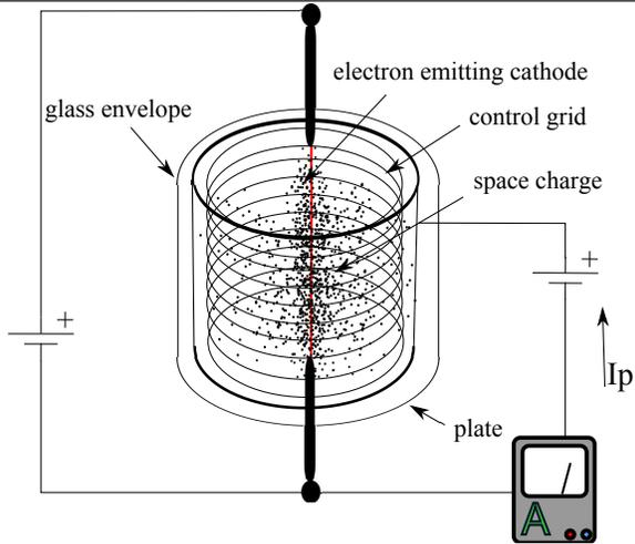
Figure 3: Electron flow inside tube.
