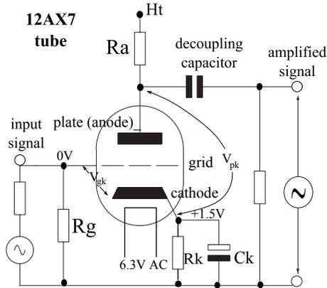
Figure 2: Common cathode circuit.
