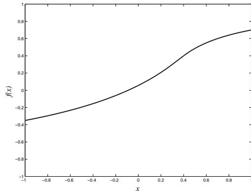
**Figure 10:** Asymmetric waveshaper proposed by Gallo [18]
