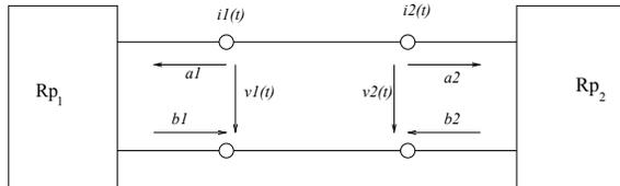
**Figure 14:** Wave Digital Filters Signal Propagation of Kirchoff Variables
