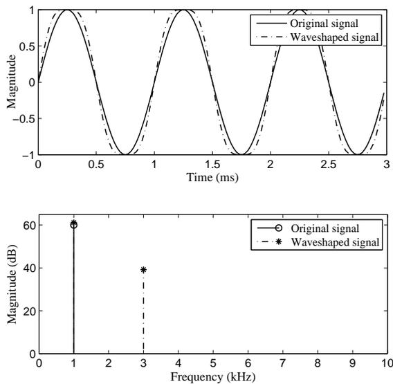
**Figure 6:** A 1 kHz sine wave filtered by Eq. 1 in the time and frequency domains.
