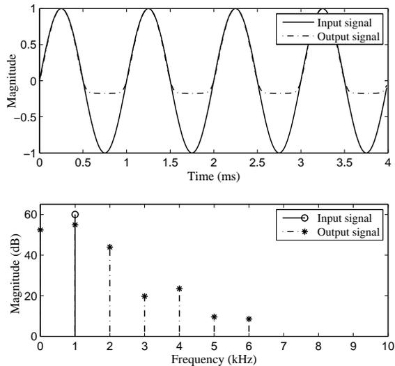
**Figure 13:** A 1 kHz sine wave filtered by Eq. 5 in the time and frequency domains.
