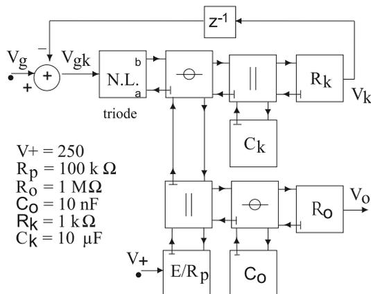
**Figure 15:** Symbolical Network representation of the first Wave Digital Filters triode models by Karjalainen and Pakarinen[24].
