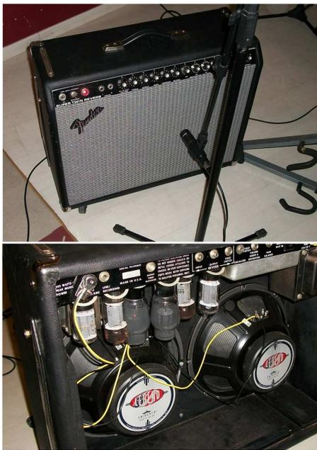
Figure 1: All tube: Fender super twin amplifier.
