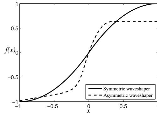
**Figure 7:** Symmetric and asymmetric waveshapers proposed by Doidic et al. [10].
