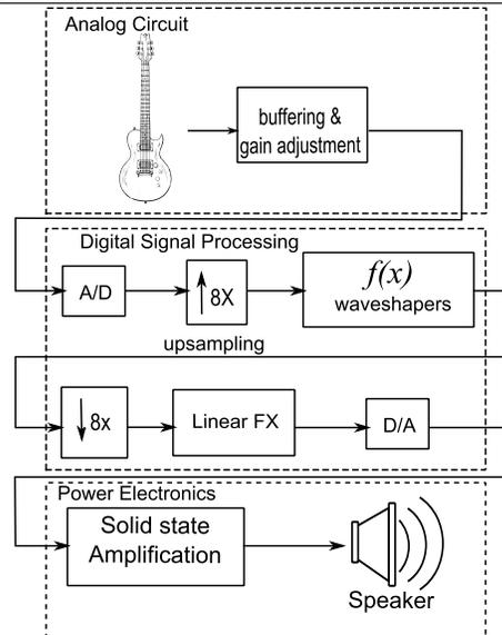
**Figure 12:** Block diagram of a DSP system for simulating vacuum-tube amplifiers [10].
