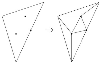
Figure 4: Hierarchical Delaunay Triangulations.
