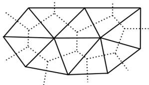
**Figure 6:** A single Delaunay Triangulation and its dual the Voronoi Diagram.
