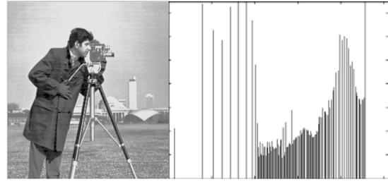
Fig. 2(f) Result of WTHE with  $r=0.5$  and  $v=0.9$  and its histogram
