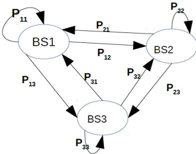
Figure 2: State transition diagram of Markov Chain with 3 BSs
