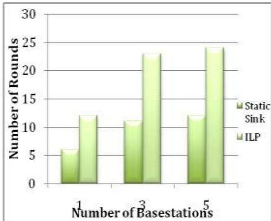
Figure 3: Network Lifetime with 200 Sensor nodes
