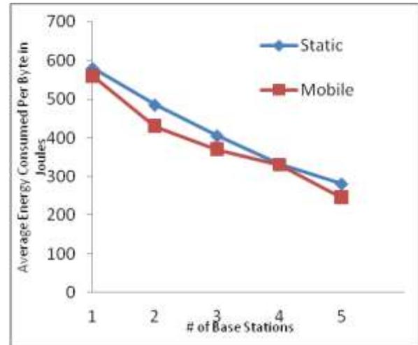
Figure 5: Energy consumption in Network with 200 nodes
