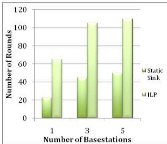
Figure 11: Network Lifetime with 100 Sensor nodes (Until the expiry of 10 % of sensor nodes)
