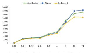
Figure 3: Number of packets sent by each node (1 Sensor)
