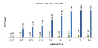
Figure 11: Injected and amplified traffic (5 Sensors)
