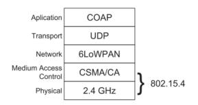
Figure 1: IoT protocol stack. Adapted from [18].
