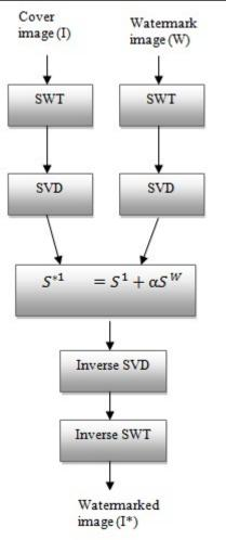
Figure 2: Block Diagram of the proposed watermark embedding algorithm
