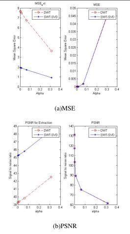
Figure 6: Comparison of PSNR and MSE for various values of scaling factor  $\alpha$ .
