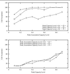
Figure 7: Call Acceptance vs. Constraints (Node Capacity and Node Association Capacity)
