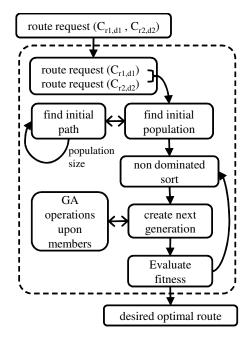
Figure 5: Workflow for finding Optimal Route
