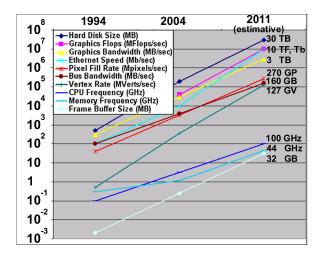
Figure 1: Various aspects of commodity hardware evolution and tendency for a single processing node equipped with a top generation Graphics Processing Unit. Except for the network speed data, all the data were extracted from Fernando's seminar [19].
