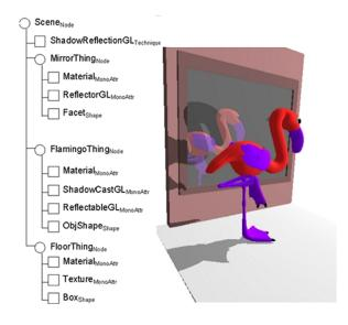
Figure 10: Example of a scenegraph defined with the *Generalized Scene Graph API* [15]. The hierarchical structure of the graph provides eased handling of complex scenes via propagated operations along the paths of the graph. Reproduced with permission granted by Jürgen Döllner and Klaus Hinrichs.
