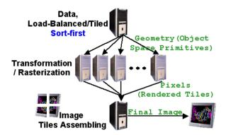
Figure 5: Classical sort-first configuration. Based on tiled partitioning information, the data is distributed among the processing nodes. After transformation and rasterization, a final step assemblies the tiles to form the image.
