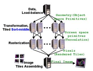
Figure 6: Sort-middle configuration with two levels of processing nodes. The screen-space data communication may also occur in between nodes at the same level, determining a one-level-only structure, where transformation nodes also act as rasterization nodes.
