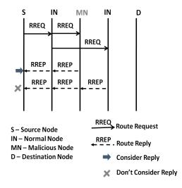
Figure 4: Route discovery in AODV in presence of attacker
