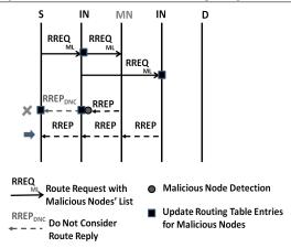
Figure 5: Route discovery in R-AODV in presence of attacker
