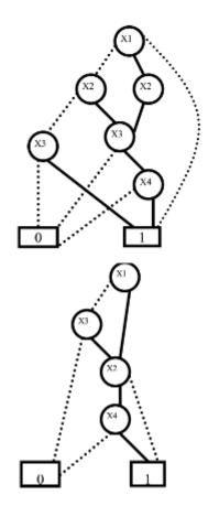
**Figure 2:** Two BDDs representation of the function  $(x1 \lor x3) \land (x2 \Rightarrow x4)$ , in the top the order of variable is: x1, x2, x3, x4; and in the bottom the order is: x1, x3, x2, x4
