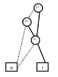
Figure 1: Binary Decision Diagram for the Boolean function f = x1x3 + x2x3
