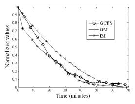
Fig. 5. Fuzzy granular index activity (GCFS) vs. Gravimetric measurement (GM) and Inertia Moment (IM)
