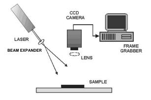
Fig. 7. Experimental set up: The lens in broken lines and the beam expander are included only for the coin image experiment.
