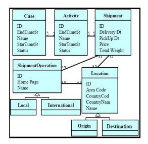
**Figure 5:** A portion of the WebML data diagram used by the Shipment Web application.
