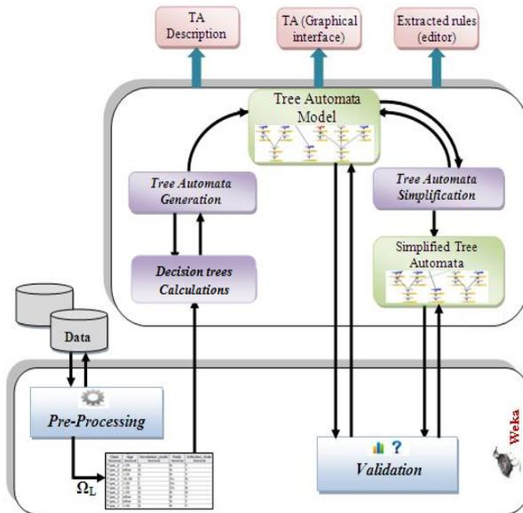
Figure 2: Steps of generation and simplification of a decision tree by a tree automaton
