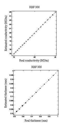
Figure 8: The evaluation vs real values of the conductivity and the thickness on the test set (+) per RBF NN
