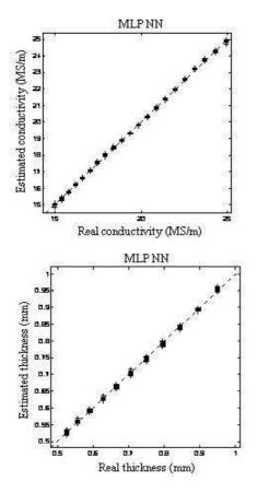
Figure 9: The evaluation vs real values of the conductivity and the thickness on the test set (+) per MLP NN
