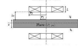
Figure 1: Geometry and dimensions of the solenoids used in method A-O for motionless sheets
