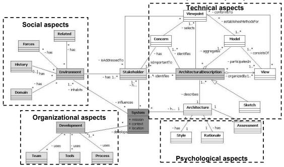
Figure 2: Software architecture meta-model (according to [3])
