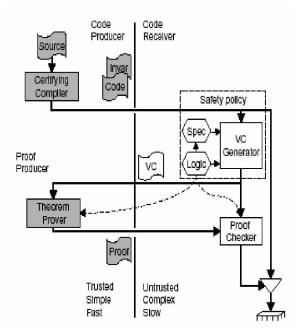
Figure 2: The basic proof-carrying code protocol. The wavy boxes represent data and code and the rectangular boxes represent system components. The white elements are trusted, while the grey elements are not trusted. [2]
