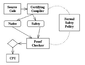
Figure 1. The basic PCC architecture
