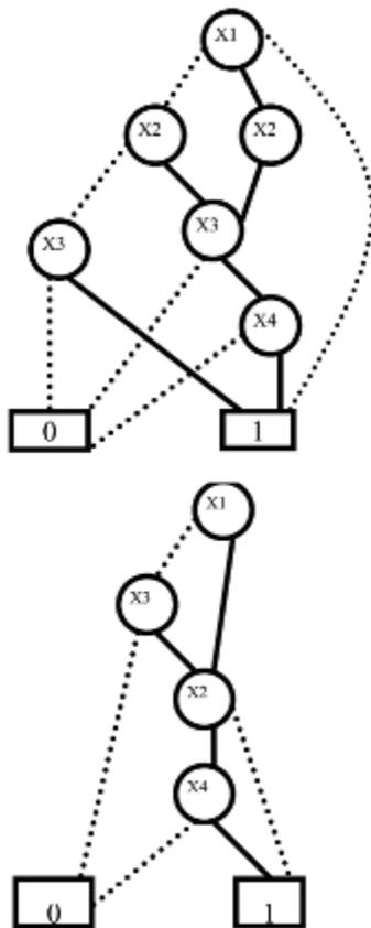
**Figure 2:** Two BDDs representation of the function  $(x_1 \vee x_3) \wedge (x_2 \Rightarrow x_4)$ , in the top the order of variable is:  $x_1, x_2, x_3, x_4$ ; and in the bottom the order is:  $x_1, x_3, x_2, x_4$
