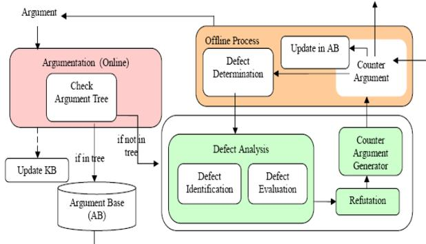
Fig. 1. (a) Prediction of Counter-arguments – Block diagram
