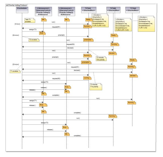
Figure 3: Sequence diagram showing deadlock avoidance using Table 1
