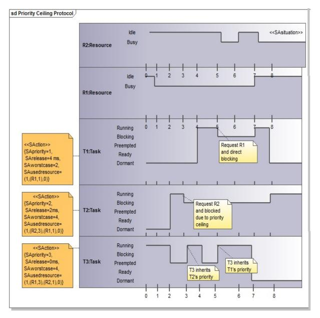
Figure 4: Timing diagram showing deadlock avoidance using Table 1
