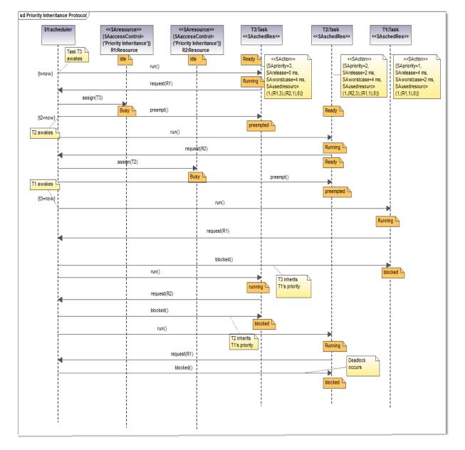
Figure 1: Sequence diagram showing deadlock occurrence using the example task set given in Table 1
