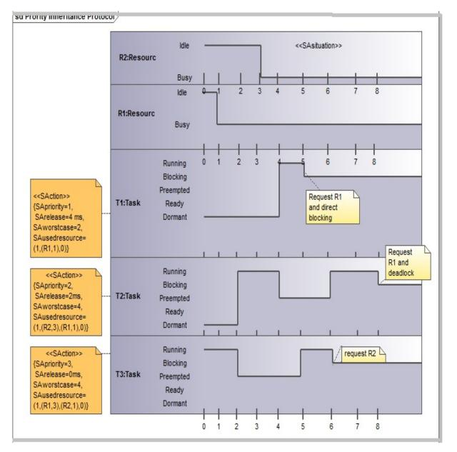
Figure 2: Timing diagram showing deadlock occurrence using the example task set given in Table 1
