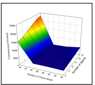
Figure5: Communication Overhead in proposed scheme with varying number of agents and number of Cluster heads
