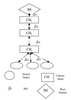
Figure4: Data Aggregation at various levels in Hierarchical Form
