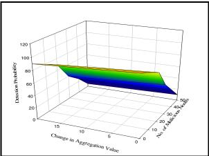
Figure7: Impact of change in count and malicious nodes on detection probability
