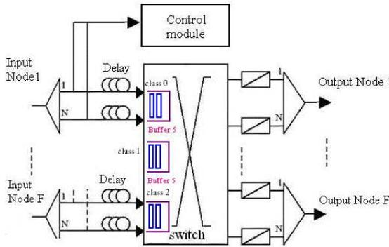
**Figure 1:** Architecture of the Optical Packet Switching Network
