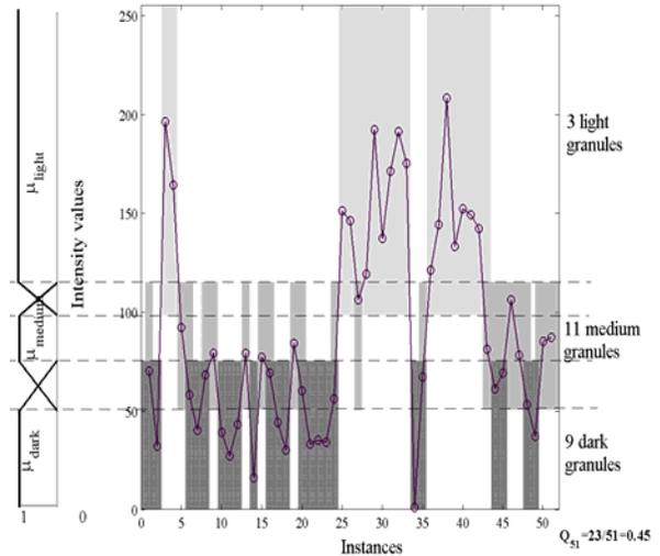
Fig.3. Methodology graphic demonstration. (Reprinted from Signal Processing, A.L .Dai Pra, et al., Evaluation of laser dynamic speckle signals applying granular computing, Signal Process 89 266–274, Copyright (2009), with permission from Elsevier.)
