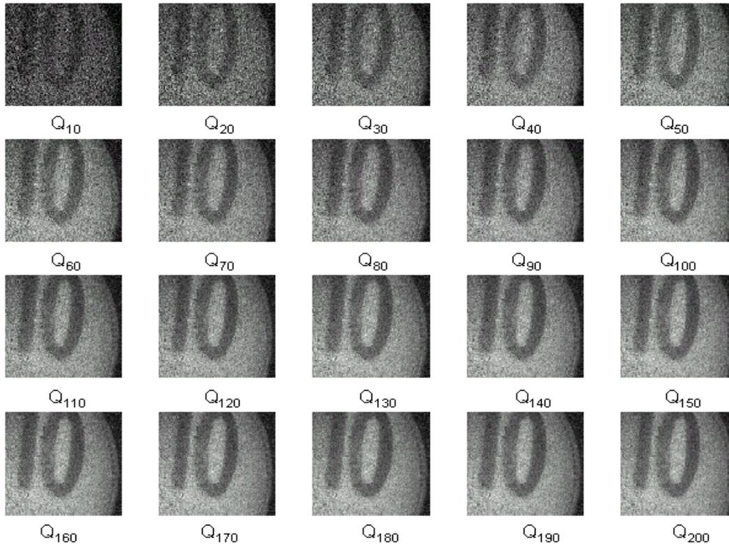
Fig. 9. Progressive sequence of activity images started from the first speckle pattern. The number under each subimage indicates the quantity of processed frames.
