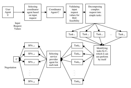
Figure 2(b): SWS Composition System with coordinator agent, which also perform some tasks
