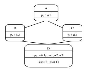
Figure.1 Class Inheritance Tree
