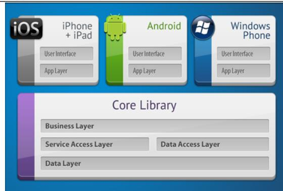
Figure 1: Architecture of multiplatform mobile application (adopted from [17]).
